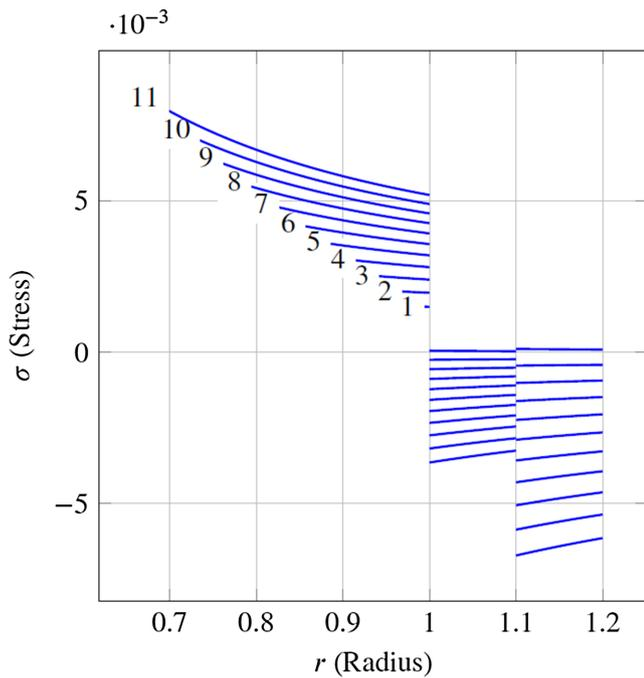
**FIGURE 10**  $\sigma_{\phi\phi}$  at the different times,  $\alpha_1 = 1$ ,  $\alpha_2 = 2$ ,  $R_1/R_0 = 1.1$ ,  $R_2/R_0 = 1.2$
