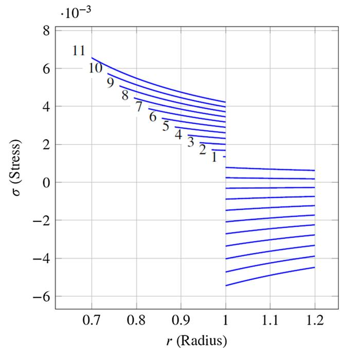
In Figure 8, the change in the magnitude of the circumferential stress on the growth surface is presented depending on the choice of Young's modulus for the cylinder. Based on the data obtained from the numerical simulations of boundary value problems, one can conclude that the stresses on growing surface have the similar time plots. The following formula allows us to approximate results by a simple scaling equation
