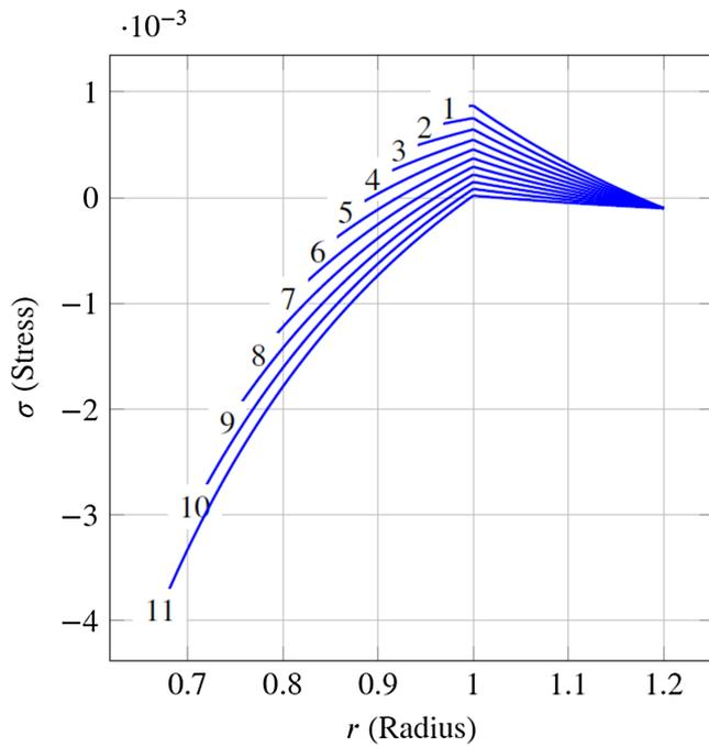
**FIGURE 2**  $\sigma_{rr}$  at the different times,  $\alpha_1 = 1$ ,  $R_1/R_0 = 1.2$
