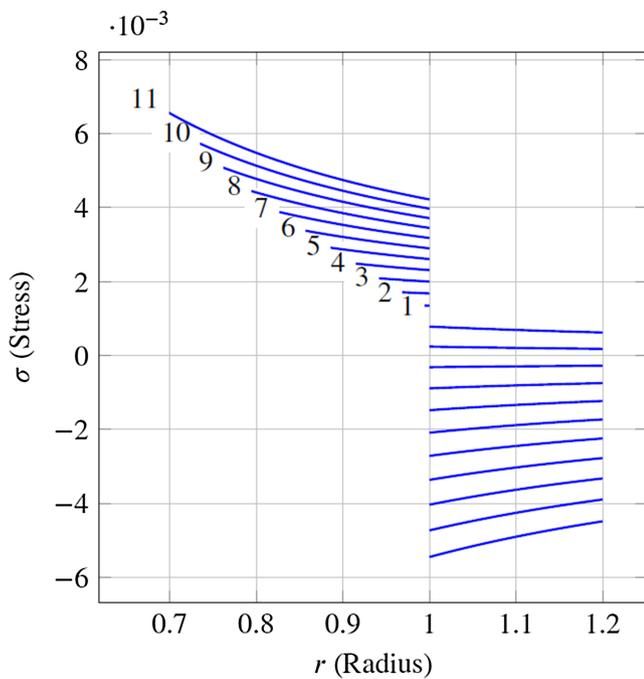
FIGURE 7  $\sigma_{\phi\phi}$  at the different times,  $\alpha_1 = 0.5, R_1/R_0 = 1.2$
