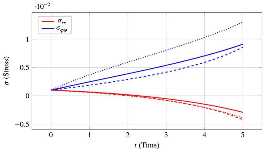
**FIGURE 1** Radial  $\sigma_{rr}$  (red lines) and circumferential  $\sigma_{\varphi\varphi}$  (blue lines) stresses on the free growing surface for  $\alpha_1 = 1$  (solid line),  $\alpha_1 = 2$  (dashed lines),  $\alpha_1 = 0.5$  (dotted lines)
