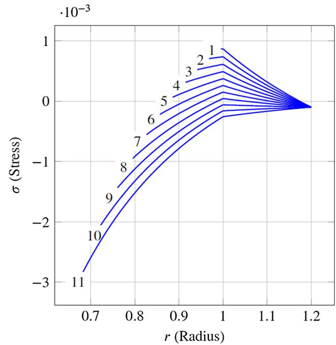
**FIGURE 5**  $\sigma_{\varphi\varphi}$  at the different times,  $\alpha_1 = 2$ ,  $R_1/R_0 = 1.2$
