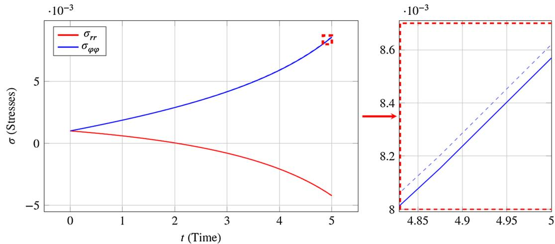
**FIGURE 11**  $\sigma_{rr}$  and  $\sigma_{\varphi\varphi}$  on the free growing surface for one-layer cylinder ( $\alpha_1^* = 2$ ) and two-layer cylinder ( $\alpha_1 = 1$ ,  $\alpha_2 = 3.2$ , dashed lines)
