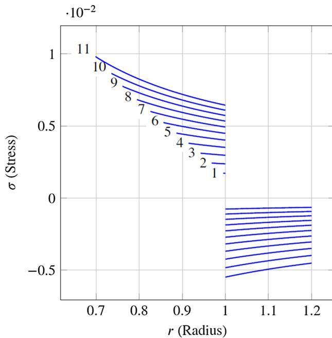
**FIGURE 3**  $\sigma_{\varphi\varphi}$  at the different times,  $\alpha_1 = 1$ ,  $R_1/R_0 = 1.2$
